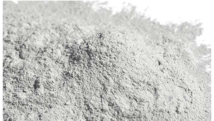
Img. 2: Glass powder from solar module recycling (Butenhoff Werbeagentur & Verlag).
