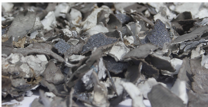
Img. 6: Recovered plastics from a solar module, including backsheet, ready for recycling (Butenhoff Werbeagentur & Verlag).
