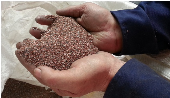
Img. 5: Recovered metal from the copper cabling, ready for re-working in the metal industry.
